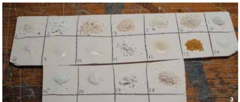
1 Bryan Hopkins' pendant lights, 7½ in. (19 cm) each, low-fire porcelain, stains, fired to cone 04 in an electric kiln, 2014. 2 Failed tests and melted pieces in the electric kiln. 3 Material tests of various raw chemicals, fired to cone 05 in an electric kiln.
